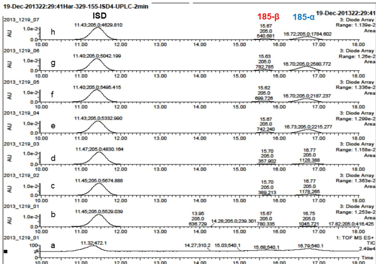
**Figure 41.** ESI-MS Coupled UPLC Analysis of Kinetic Experiments as Illustrated for the Pseudo-first-order Kinetic Experiment with Respect to the Donor ( $0.056 \text{ mol dm}^{-3}$ ) and Acceptor ( $0.034 \text{ mol dm}^{-3}$ ); <sup>a</sup>ESI-MS trace at  $t = 2 \text{ min}$ ; <sup>b-h</sup>TUV traces at different time points.
