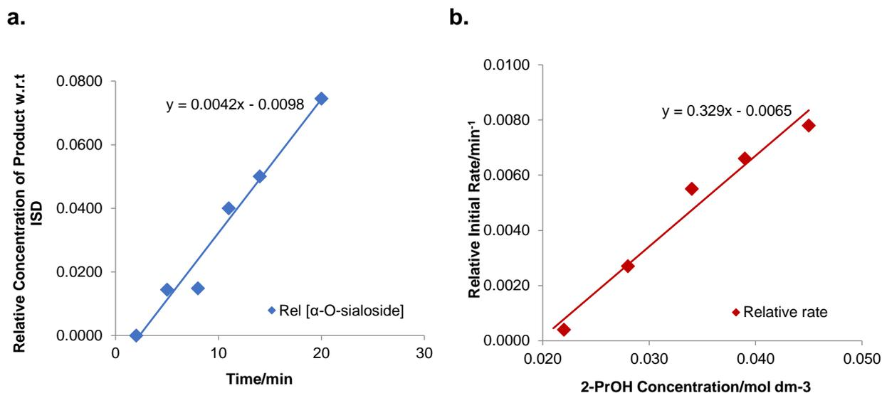
**Figure 42.** The Influence of Acceptor Concentration on  $\alpha$ -O-Sialidation of  $\beta$ -Thiosialyl Donor **183 $\beta$** ; **a.** Relative Concentration of Product w.r.t. Internal Standard (ISD) vs time ( $[2\text{-PrOH}] = 0.028\text{ M}$ ) and **b.** Relative Rate vs Concentration of 2-PrOH.
